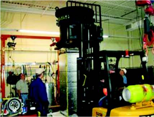
Researchers and staff at UT's Magnet Development Laboratory prepare the central solenoid mockup for the vacuum pressure impregnation process. (Credit: University of Tennessee, Knoxville)
